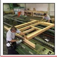
Now a good share of new homes are built in factories and delivered to the home site and assembled. This includes roof trusses, cabinets, doors, flooring, windows, and even walls. Our fireplace mantle was delivered and assembled in a couple of hours instead of having a carpenter spend days building it on site.
